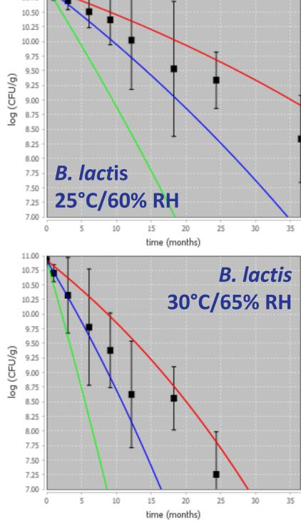
Long-term stability data (error bars  $\pm 1\sigma$ ) for cell viability (log (CFU/g)) of capsule products packaged in 100-cc HDPE (HIS) bottles containing 60 capsules and 1 g of silica gel desiccant overlaid on loss predicted by ASAP*prime*<sup>®</sup>. Blue line: mean predicted behavior. Green and red lines: 90% confidence interval.
