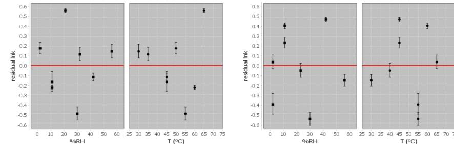
Residuals plots of fit to the Arrhenius model for loss of cell viability in *L. acidophilus* (left) and *B. lactis* (right) powder
